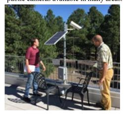
USGS to further develop and field deploy one particular element of FloodAware: the solar-powered, cell-connected smart cams we invented that can be cheaply and easily installed to monitor for flooding anywhere.
