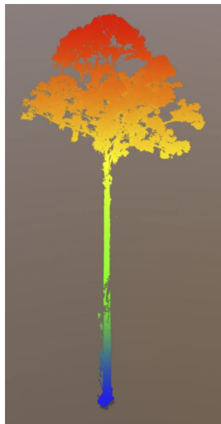
Figure 1. A 3D scan (combined TLS and SfM) of the world's tallest tropical tree.
