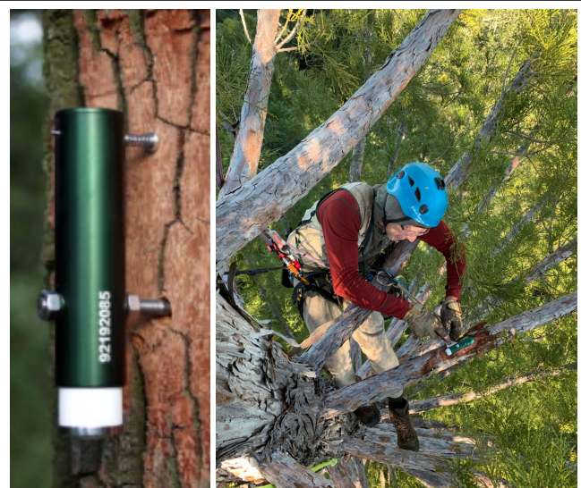
Left: miniature TOMST dendrometer. Right: Prof. Koch installing a dendrometer at the top of a 300' high coast redwood in California.
