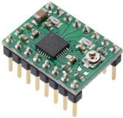
Figure 26- Ball-on-Beam Prototype: Stepper Driver
