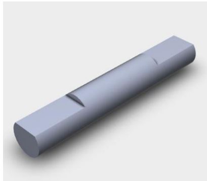
Figure 24: Interior beam segment with machined lips
