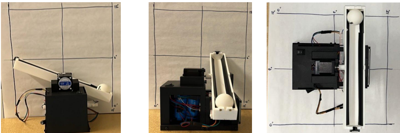
Figures 41-43: Left to Right - Profile, Front, and Top views of Robot #1 Verifying dimensions under 12 inches
