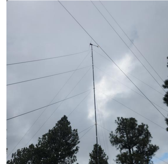
Figure 4: Cup Anemometer at RE Lab \sim 90 ft from ground
