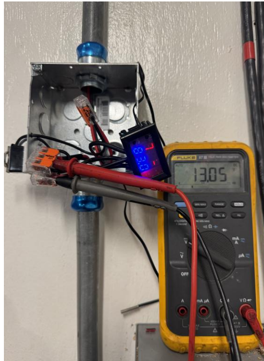
Figure 9: Multimeter Voltage Test at First J-Box
