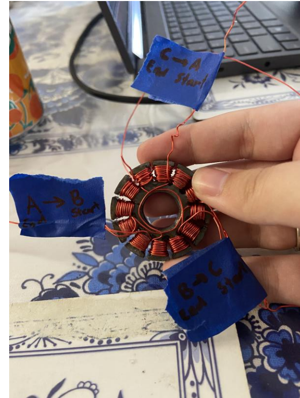
Figure 14: Completed Winding Back
