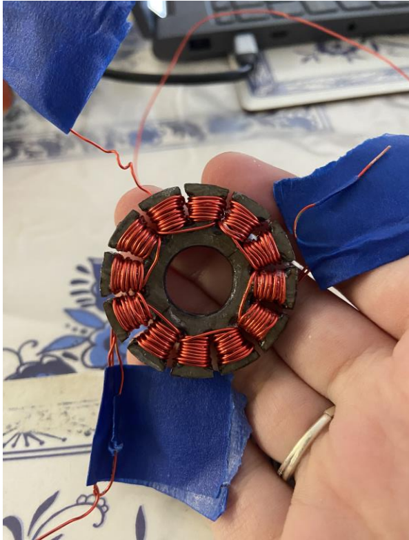
Figure 13: Completed Winding Front
