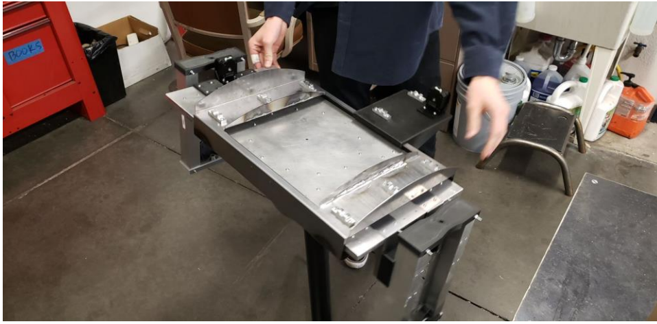
Figure 7: System with Z Carriage and Y Axis Rails Subsystems Installed
