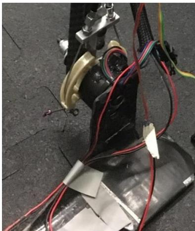
*Figure 41: intermediate design, 3D printed Pulley*
