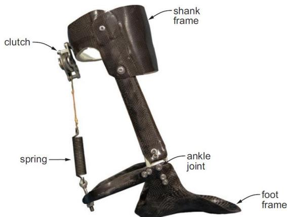
Figure 1: Sawicki Passive Device (profile view) [20]
