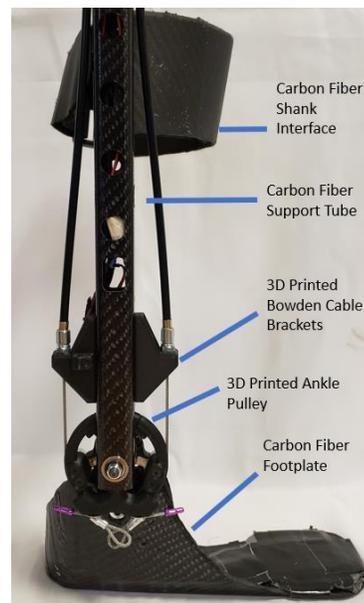
Figure 33: Optimized lower leg assembly
