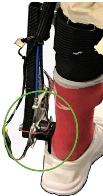
Figure 35: moment arm, COTS torque sensor, cantilevered design [34]
