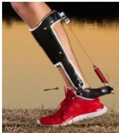
*Figure 11: Passive Exoskeleton with significant Posterior Protrusion [32]*
