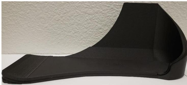
*Figure 57: interlocking 3D printed footplate molds*
