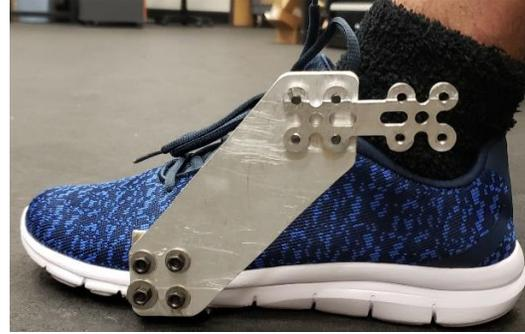
*Figure 30: strut design foot interface*
