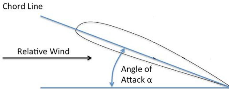
Figure 4: Angle of Attack for Rotor Blade Design [5]
