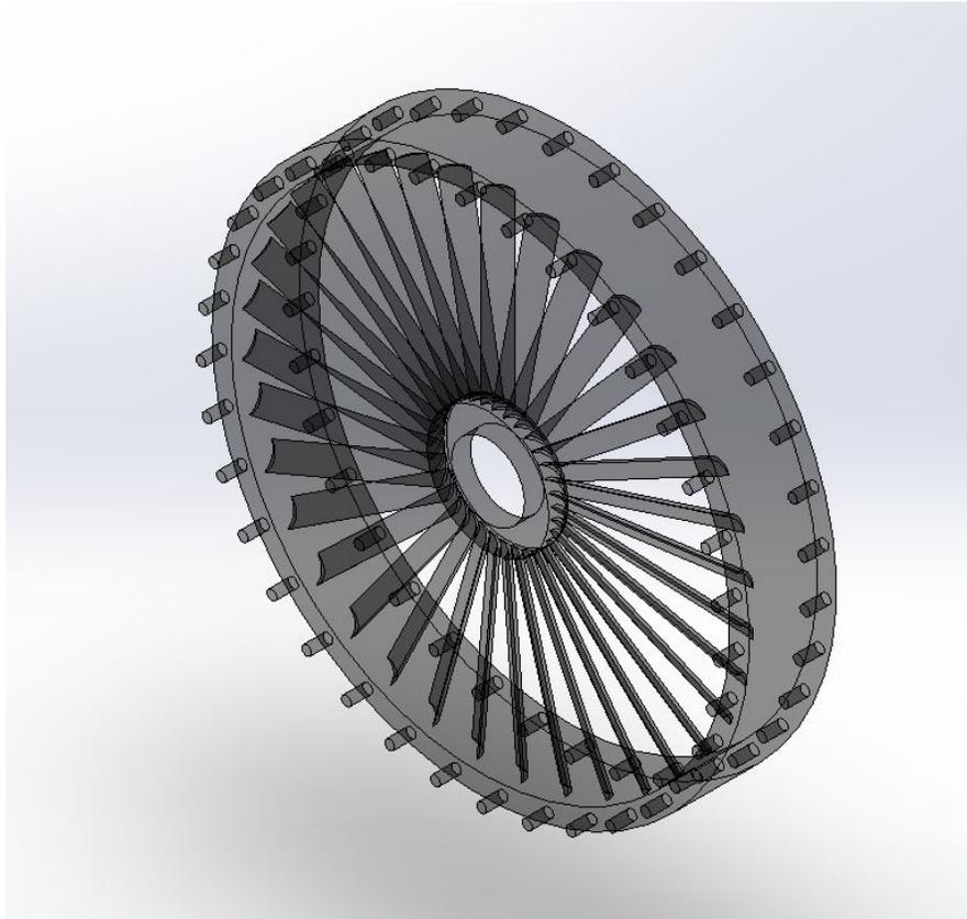
Figure 22: Stator Structure
