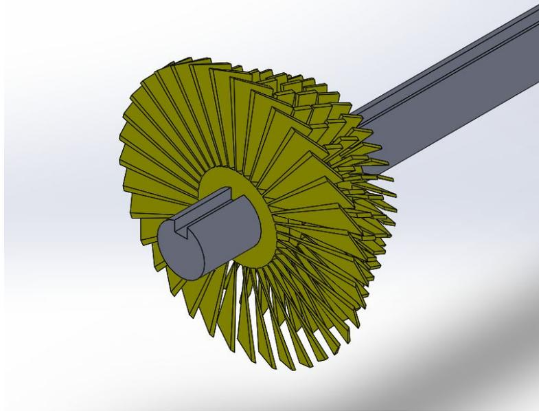
Figure 16: Compressor Cascade
