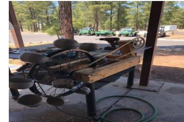
Figure 4: Water Wheel Turbine
