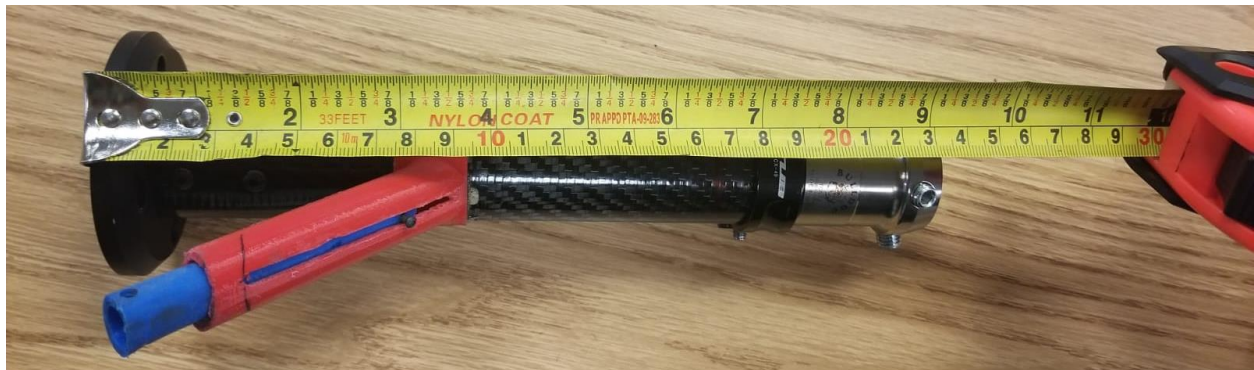
Figure 1: Pylon at short state
