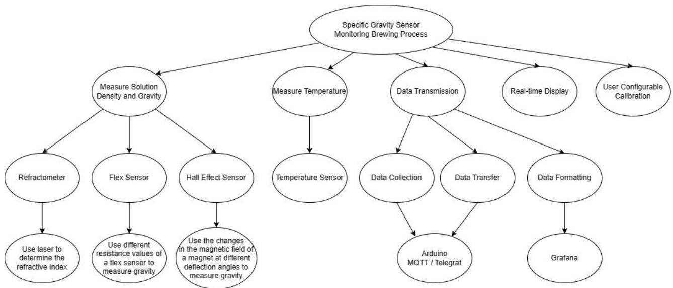
In the functional analysis of our project, the primary function of the system is the precise measurement of the specific gravity and temperature of the liquid during brewing, with real-time
