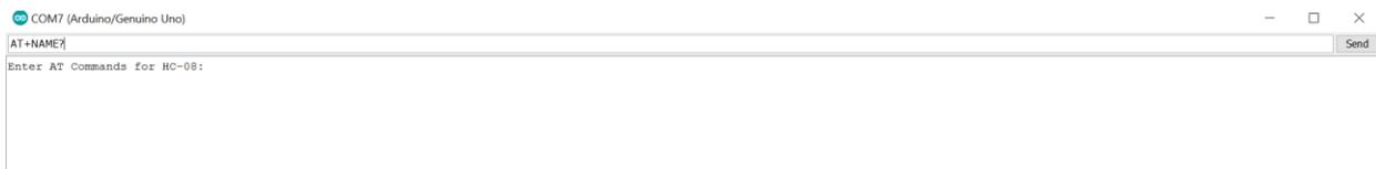
After clicking on Send (or pressing enter), The screen will read “Enter AT Commands for HC-08:” a new line will appear. This line will say “OK+Name: ” and the name of the module. In this case it showed “OK+Name:SH-HC-08”, which is the name of the module used to create the guide is SH-HC-08. The name of the module is the name of the Bluetooth device you want to connect to when you connect with the mobile application.
