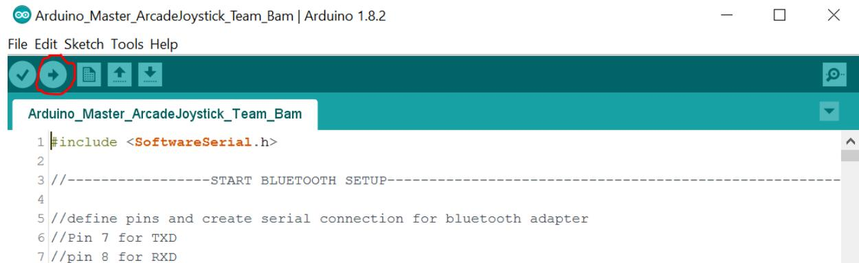
**Step 10:** After the green bar disappears from the last step the Arduino is now ready to be used with the Arcade style joystick to control the car. Follow these steps for flashing the code for other control devices, just choose the appropriate file for that controller.
