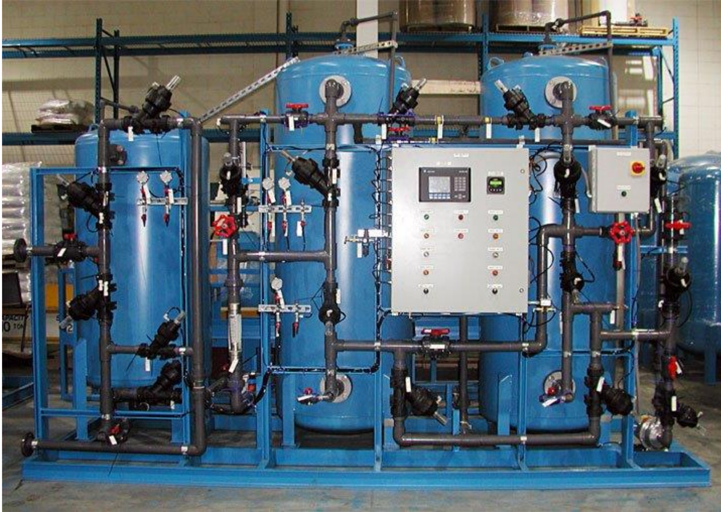
Figure 10: Industrial Mixed-Bed Deionizer from Industrial Water System
