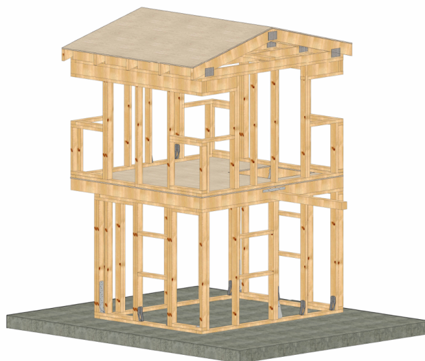
Figure 6: Structural View BIM Model
