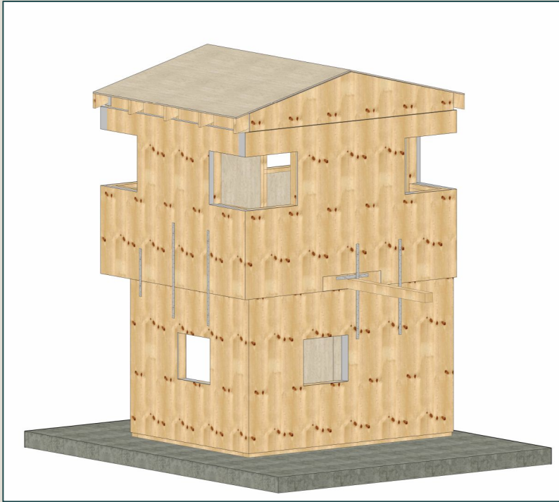
Figure 12: Exterior Sheathing 3D View [5]
