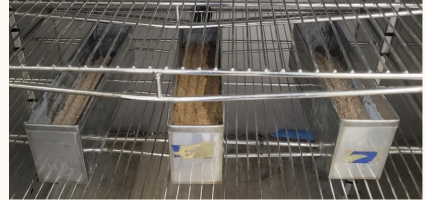
Figure 10: Soil Troughs in Drying Oven
