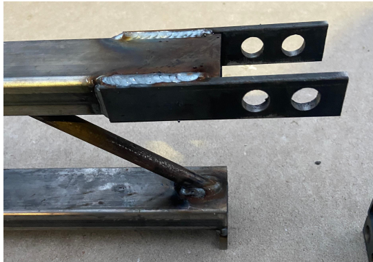
Figure 31, Incorrectly Fabricated Connection
