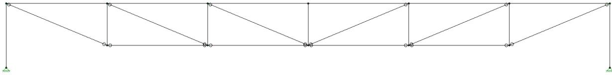
Figure 2-3: Underslung Howe Truss Alternative Elevation View
