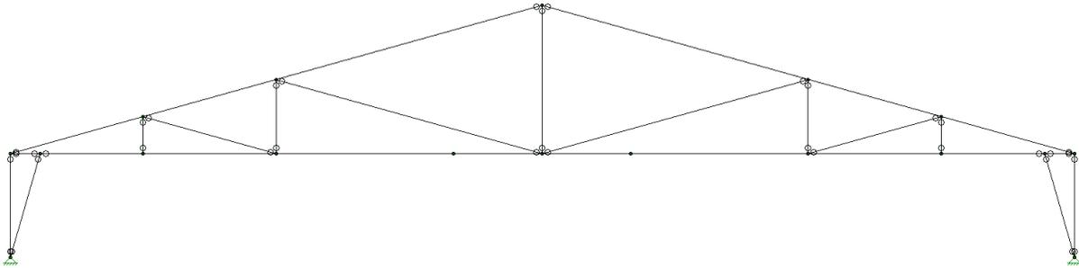
Figure 2-1: Double Howe (KK) Truss Alternative Elevation View
