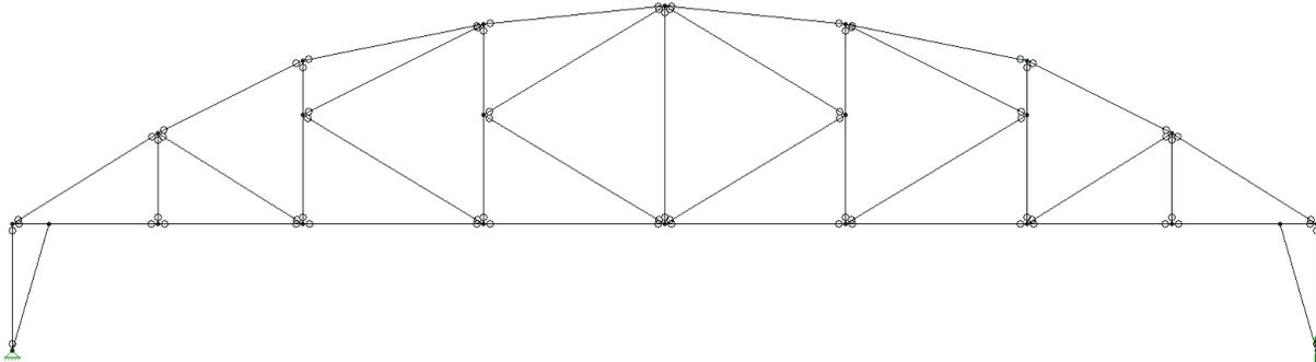
Figure 2-2: Parker (K) Truss Alternative Elevation View
