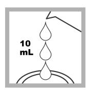
7. Prepare the blank: When the second timer expires, fill a second sample cell with 10 mL of sample.
