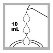
7. Prepare the blank: When the second timer expires, fill a sample cell with 10 mL of sample.
