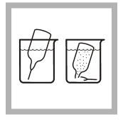
3. Tap the bottom of a NitraVer 5 Nitrate AccuVac Ampul to dislodge the powder. Fill the Ampul with sample. Keep the tip immersed while the Ampul fills completely.
